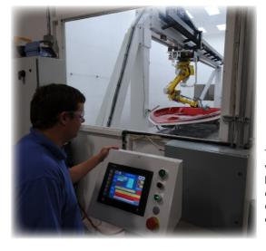
The enclosed JetTool waterjet cutting system keeps operators safely away from the trimming area while the robot is at work.
