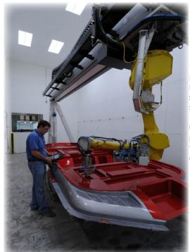
Robot programming is made easy with specialized software including KMT's TrimPro®, used for offline programming and virtual workcell creation.
